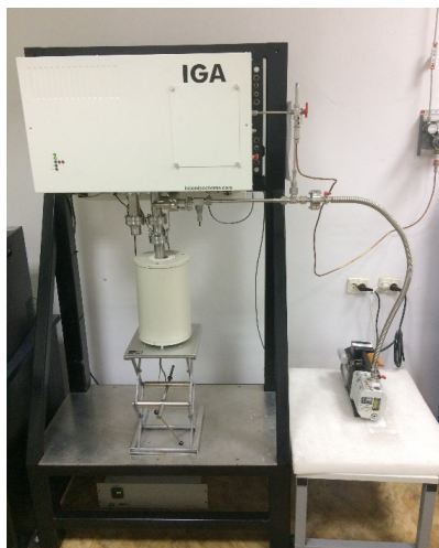
Fig. 1. IGA-001 gravimetric system for gas sorption measurements
