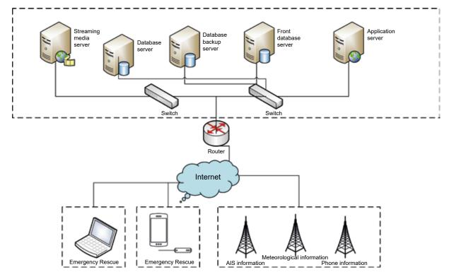
Figure 3. Hardware system composition
