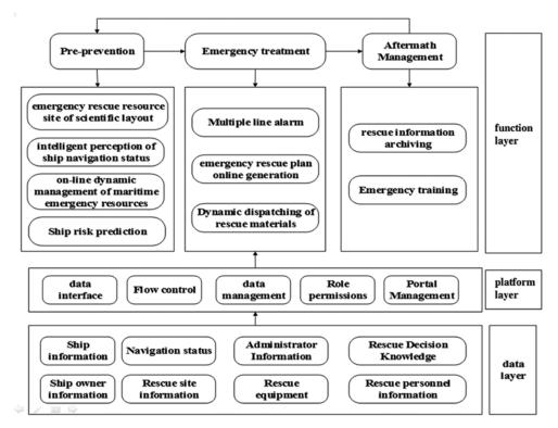
Figure 1. The platform's design framework
