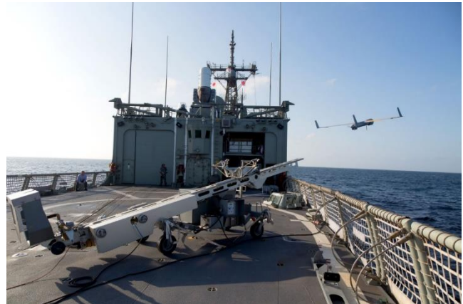
Figure 2. Photo showing the launch of the Scan Eagle UAV from the deck of the ship. In the foreground you can see an aircraft launcher. The use of airframe (UAV) on board ships requires taking into account the presence of such devices on board. Source: https://www.navy.gov.au
