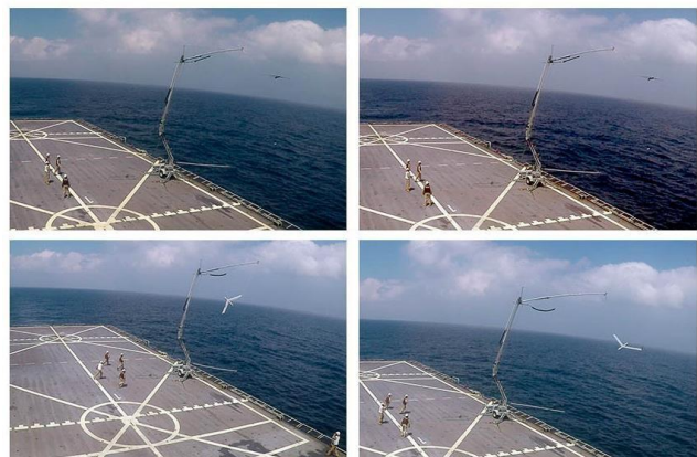
Figure 4. Scan Eagle landing sequence on board. Visible mast for intercepting the plane. After folding, the mast must find a place on the ship's deck. Source: https://www.navaltoday.com
