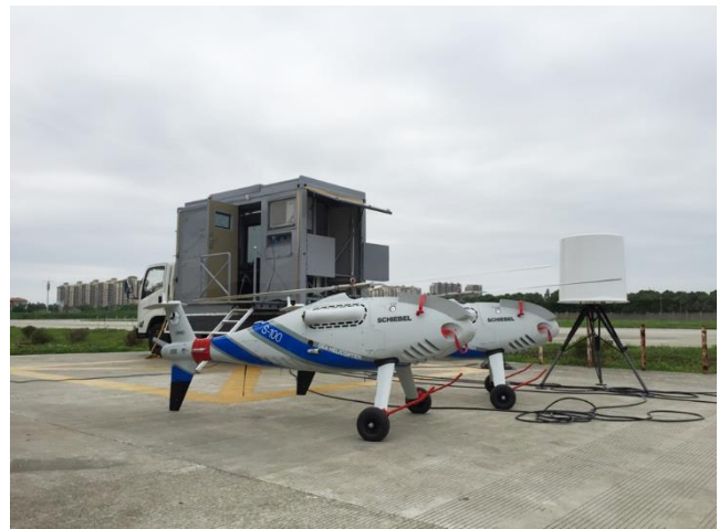
Figure 3. The Camcopter 100 drone in front of the GCS and antenna unit. Operation of the UAV from the deck must take into account the need to deploy these elements on the ship / naval ship. Source: https://penaviation.com
