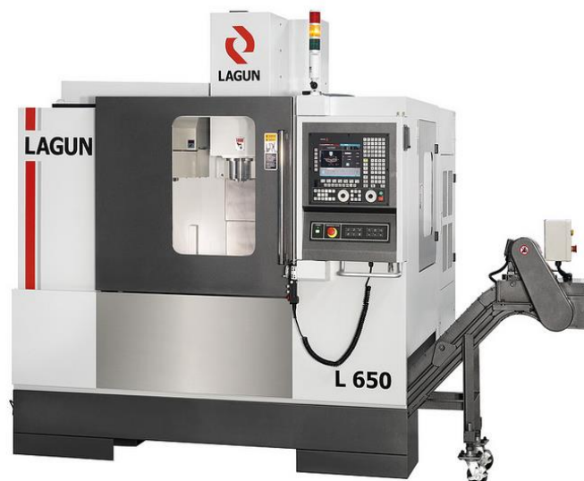
Fig. 3. Vertical machining centre with a guard
