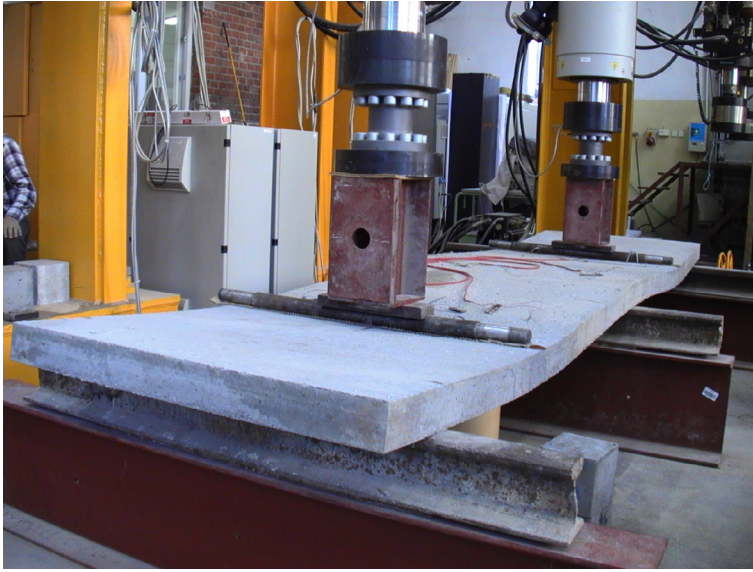
Fig. 7. Slab B-2 shortly before its failure
