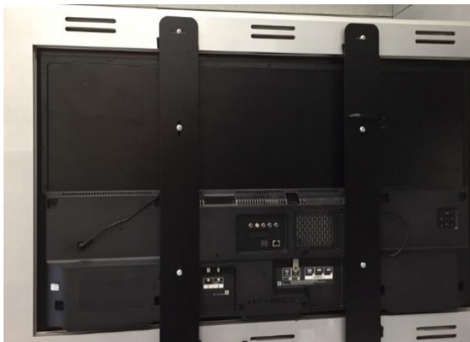
Fig. 6. A photo showing the monitor installation along with the cooling channel holes made in the wing structure. Source: authors
