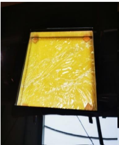
Fig. 8. Photo showing glass glued to black glossy acrylic with space for a tablet. Source: authors
