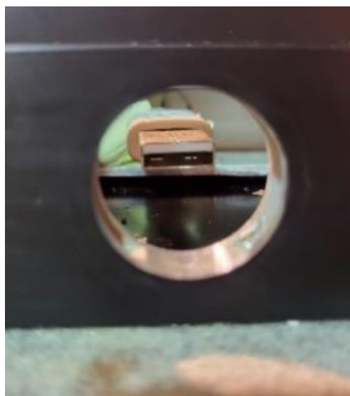
Fig. 3. Photo showing the milled hole for external connections in the leaf structure. Source: authors
