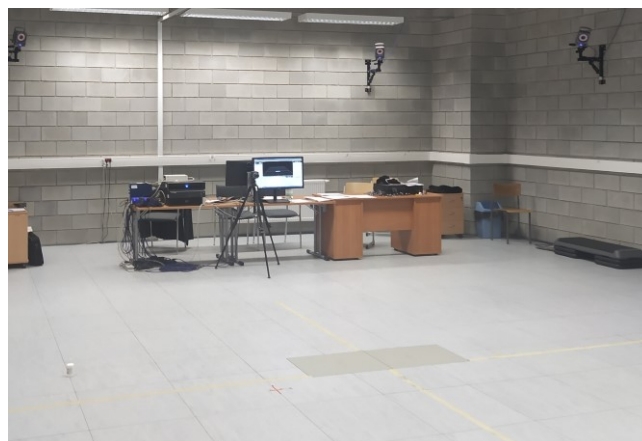
Fig. 1. Image of the LUT testing path with two AMTI-manufactured force plates indicated in the foreground. LUT, Lublin University of Technology
