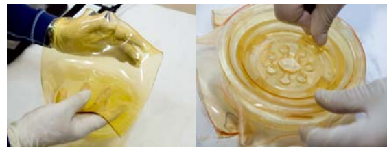
Fig. 9. Process of applying an optically active layer of real torsional vibration damper made of resin and the casting method
