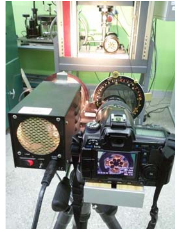
Fig. 15. The test bench along with Vishay polariscope used to analyze the stress distribution in torsional vibration damper
