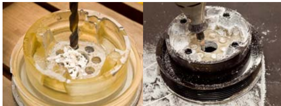
Fig. 13. Drilling of holes in the optically active layers
