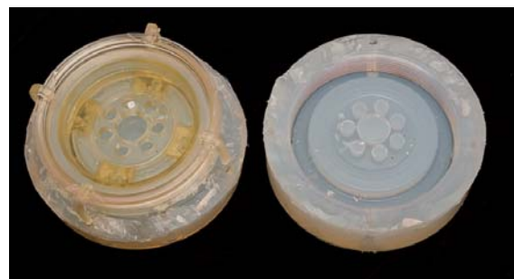
Fig. 6. Process of separation of torsional vibration damper model form
