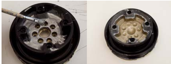
Fig. 12. Optically active layers adhered on the model of the torsion vibration damper in justified cases
