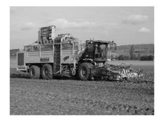
Fig. 1 6-row beet harvester – method beheading (Source: KWS, 2014)
