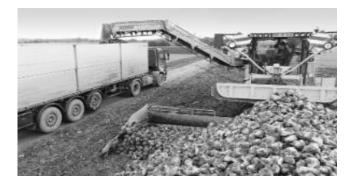
Fig. 4 Loading of sugar beets using beet cleaner loader (Source: Südzucker AG, 2012)
