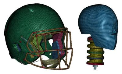
Figure 3. Discrete model of helmet and head
