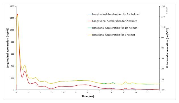
Figure 7. Resultant accelerations graph in head to head setup with both moving helmets
