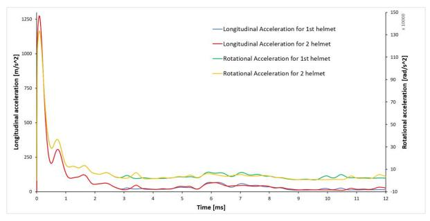
Figure 9. Resultant accelerations graph in offset setup with both moving helmets
