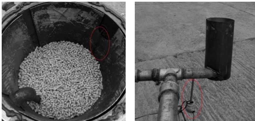
Fig. 3. Photos of the mounted sensors; TI left in the combustion chamber (shown pellets ready for gasification) to the right exhaust gas with TIV
