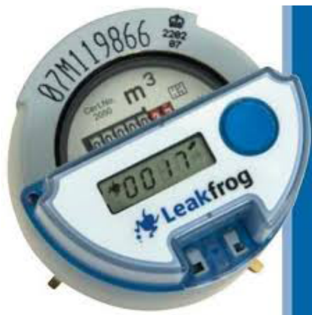
Figure 8: Leakfrog device installed on a water meter.
