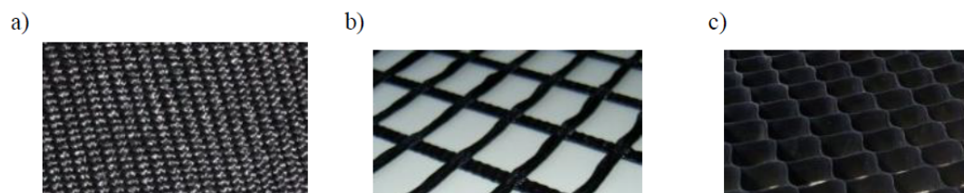
Figure 11. Types of geosynthetics: a) geotextile, b) geogrid, c) theocrat [6]
