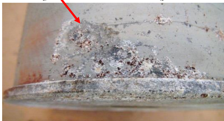
Fot. 13. Korozja łusek: a - stalowa do 122 mm naboju, b – mosiężna do 152 mm naboju Photo 13. Corrosion of cases: a – steel one for 122 mm cartridge, b – brass one for 152 mm cartridge
