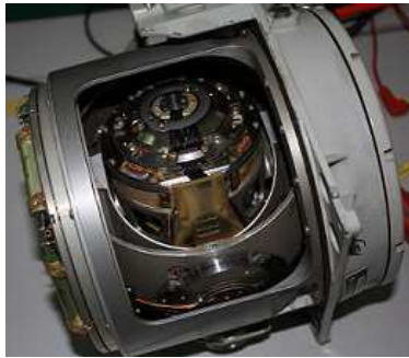
Fig. 1. The physical structure of the four-gimbal platform.
