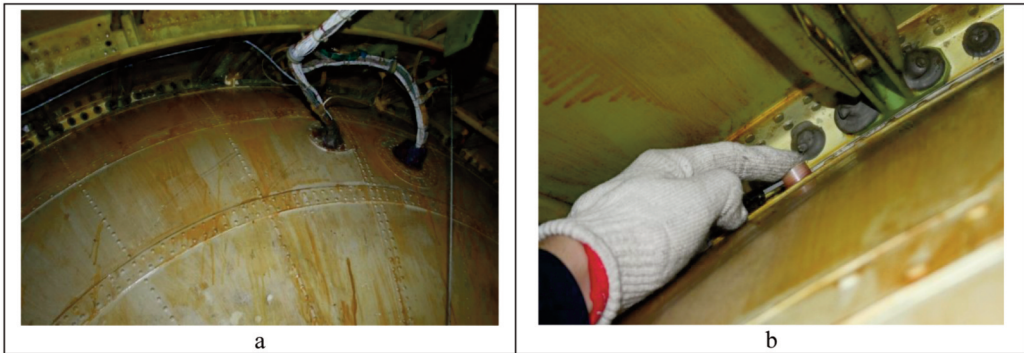
Fig. 4. Hard-to-reach bulkhead area of Boeing-747 (a) and inspection procedure of the manual placement of developed ring type EC probe on the rivet head (b).
