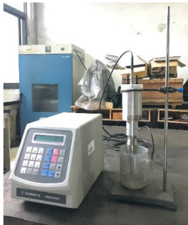
Fig. 2. Schematic of ultrasonic treatment experimental setup
