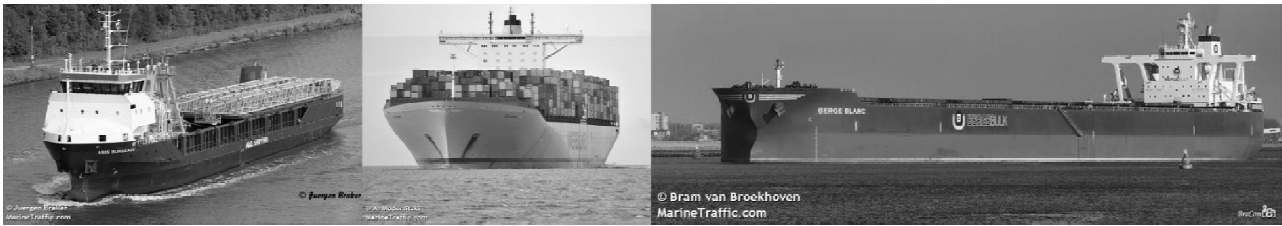
Figure 5. Illustrative photographs of vessels used for visual assessment, with the superstructure and the antennas on foredeck (left), amidships (middle), and afterdeck (right) [source: MarineTraffic.com]
