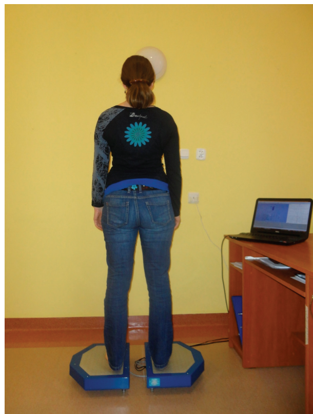
Fig. 2. Model on bi-modular stabilometric platform CQStab2P
