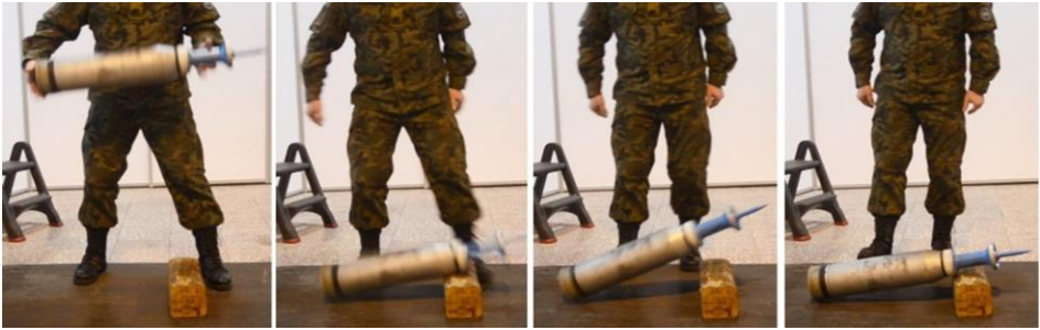
Fig. 9. Impact of a 120 mm cartridge with its case adapter against a blunt edge during a drop from approx. 1 m
