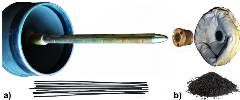
Fig. 5. Examples of propelling charge initiating components in the 120 \times 570 mm cartridge: a – DM132 igniter, integrated with a metal sleeve for the igniting charge in the form of compressed rods; b – G UW-7-120 (EZA-1) igniter and the igniting charge with the flash reducing agent packaged in a cotton bag with black powder
