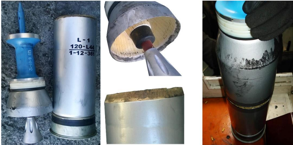
Fig. 6. Example of defective ammunition: as a result of a defective adhesive bonding process, the cartridges were partially (see right) or completely disintegrated (see left) [courtesy: Polish Armed Forces Support Inspectorate]
