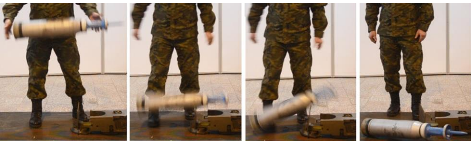
Fig. 10. Impact of a 120 mm cartridge with its case adapter against a sharp edge during a drop from approx. 1 m
