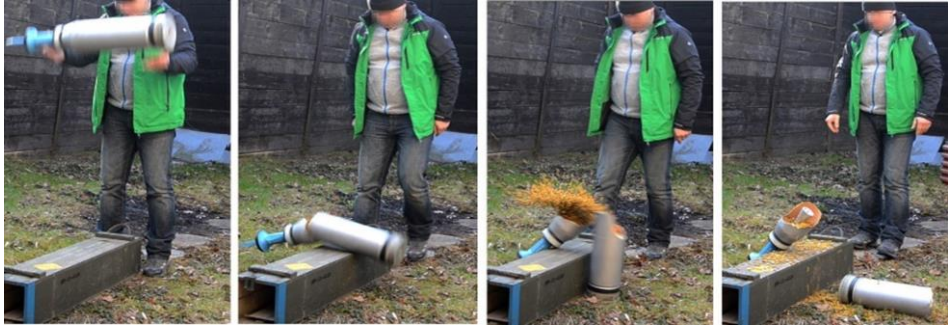
Fig. 12. Approx. 1 m high drop of a 120 mm cartridge with a part of the combustible cartridge case hitting a hard substrate
