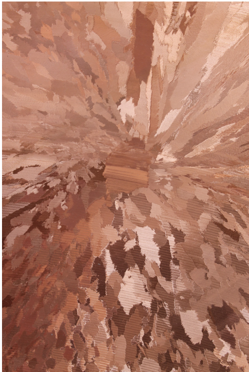
Fig. 12. Upper view of two types of the structural transitions: C>SC (columnar into single crystal transition and partially: E>SC (equiaxed into single crystal transition)
