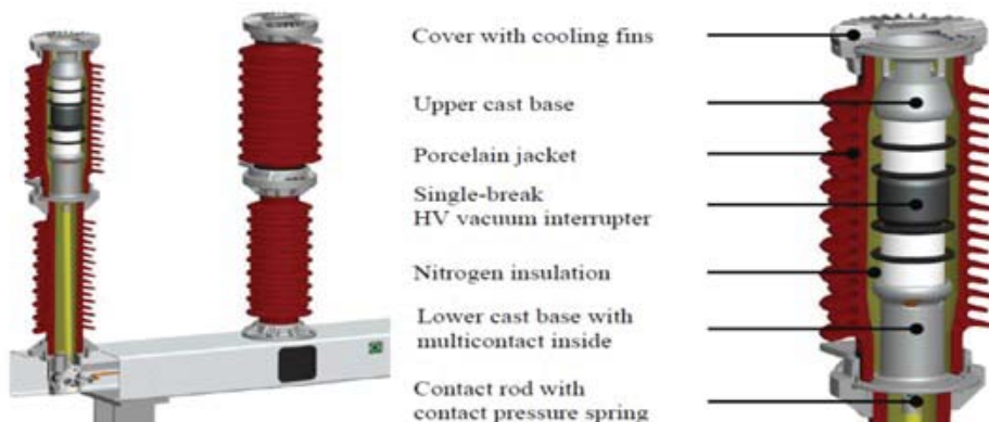
Fig. 2. Sectional view of vacuum circuit breaker pole with cross section of this pole [2]
