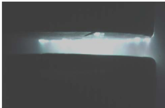
Fig. 13. Diffusion arc recorded with high speed Photron camera
