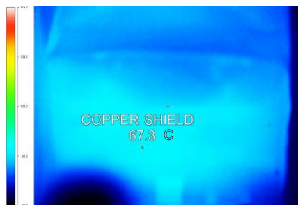
Fig. 3. Thermal image of quasi-distributed-gap PFC choke with copper shield around windings
