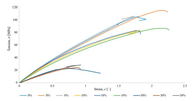
Figure 6. Static stretch test for samples with recyclate content of 0, 10, and 30%, with recyclate granulation ≤ 1.2 mm
