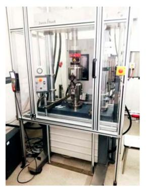
Figure 5. The universal strength machine from Zwick Roell
