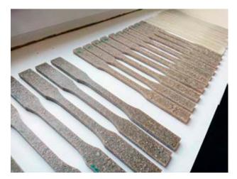
Figure 4. Samples prepared for static stretching: in the foreground a sample of 30% waste, then a sample group with 10% recyclate and clear samples without recyclate
