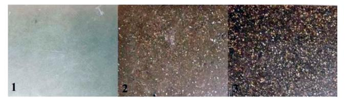
Figure 2. Hardened composite panels: 1 – without recyclate, 2 – 10% recyclate, 3 – 30% recyclate (photo taken with 13 Mpixel camera, Sony IMX 214 sensor and focal length 27 millimeters)
