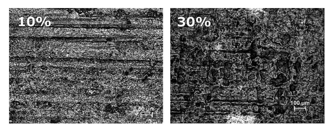
Figure7. Cross section of the composite with 10% and 30% filler
