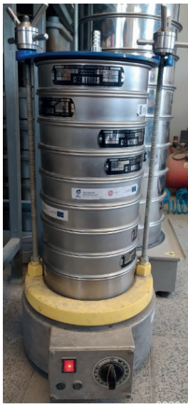
Fig. 2. Multi-level screen for abrasive grain with side vibrators station
