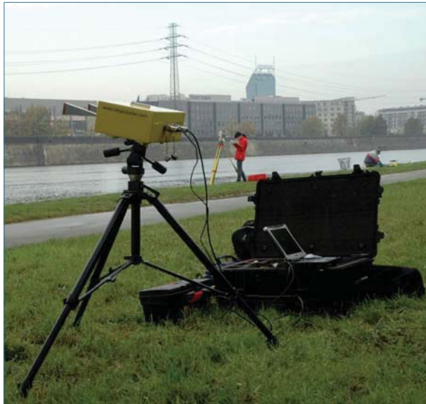
Fig. 1. IBIS-S system during measurement
