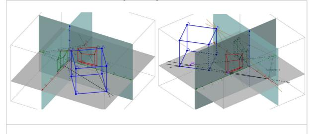
Figure 2 Left:Two central projections of a cube from two different centres. Right: Incorrectly meeting epipolar lines inside mapped cube.
