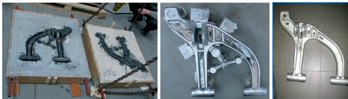
Fig. 1. The manufacturing steps of the sand casting technology: preparation of the sand mould, casting after shaking out of the mould, casting after machining and heat treatment
