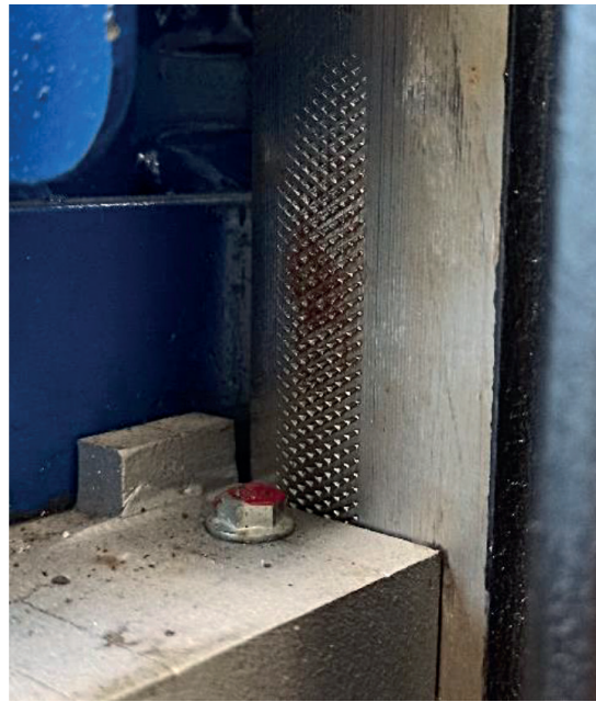
Figure 2. View of RP90/B guide rail with main dimensions and red-marked working surface S, plastic deformed guide rail surface after engaging the catcher.
