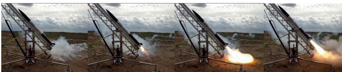
Fig. 4. Rocket motor start sequence during take-off in the field test
