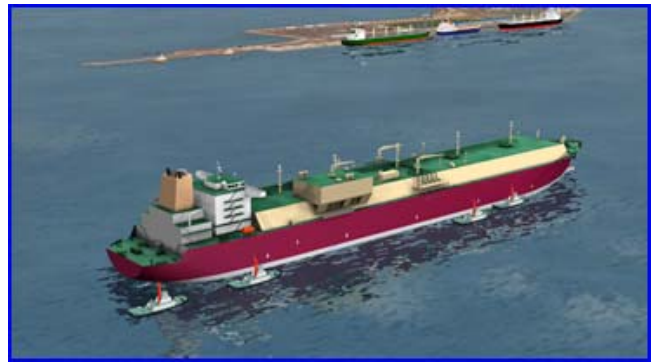
Figure 5. Computer graphics-generated image of LNG carrier used in the manoeuvring simulation tests (217K Membrane)
