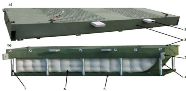
Fig. 4. Single prototype module – cassette with PCO: (a) in the closed position of the bottom plate – PCO without compressed air, (b) in the opened position of the bottom plate with PCO filled with compressed air. Designations: 1 – horizontal rod joints, 2 – cassette with roadway, 3 – vertical rod joints, 4 – module stem-deflector, 5 – bottom plate, 6 – elastic pontoon, and 7 – single telescopic mechanism
