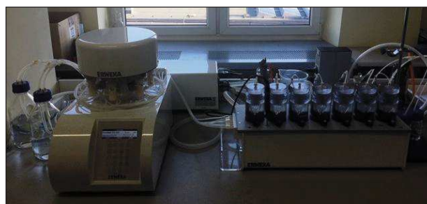
FIG. 1. The equipment used for USP4 method (DZF II Flow-Through System, Erweka GmbH, Langen, Germany).
