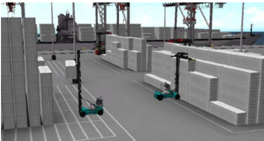
Figure 5. The equipment providing the top and side access to the stack
