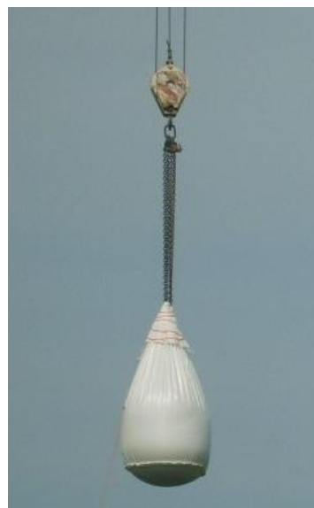
Fig. 2. Water capsule worked-out during field tests – the outer view of an actual capsule
