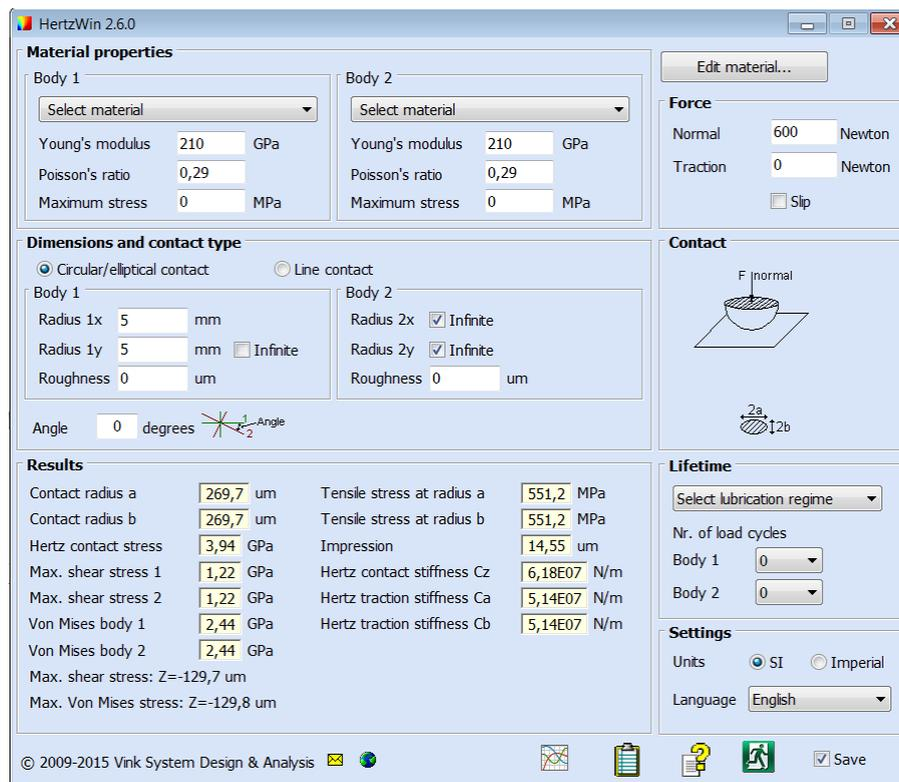
**Figure 3. The results of calculations of the program HertzWin: ball radius 5 mm, force 600 N, with Young's modulus and Poisson's ratio the same for the ball and cylindrical specimen:  $E = 210$  GPa,  $\nu = 0.29$**
