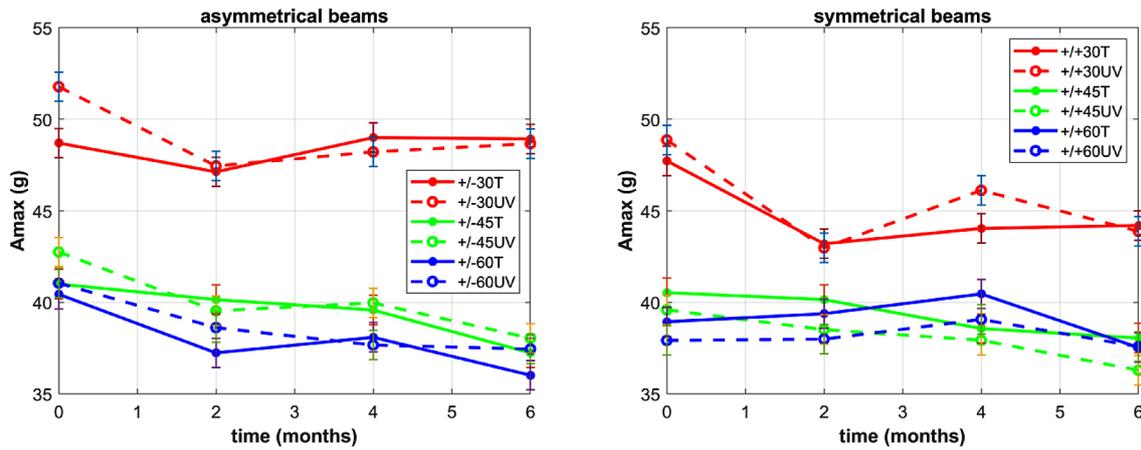
**Figure 13.** Maximal amplitude expressed by gravity acceleration (g) attained of all compared composite structure via time expressed by months periods of conditioning for asymmetric (a) and symmetric cantilever beams (b)
