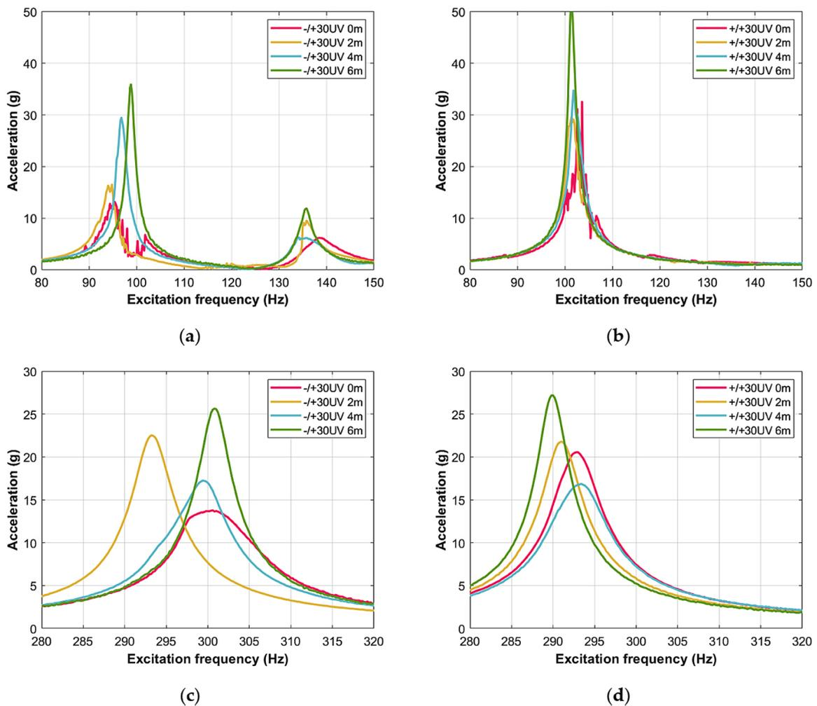
**Figure 11.** The amplitude – frequency responses of the cantilever beam with fibre set configuration 30°, exposed to UV radiation in the vicinity of the second (a, b) and the third (c, d) resonance zones, respectively
