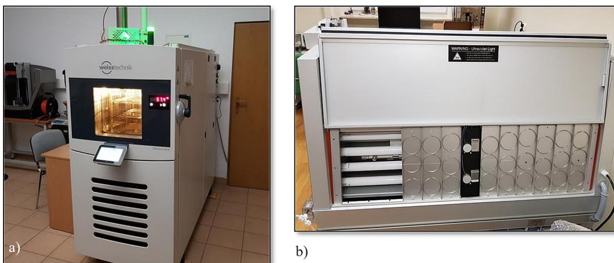
**Figure 3.** (a) Stand of the thermal shock chamber Weissttechnik used in laboratory; temperature range, hot chamber: +50°C to +220°C, cold chamber: -80°C to +70°C (b) stand of the accelerated atmospheric aging chamber QUV/SPRAY/RP
