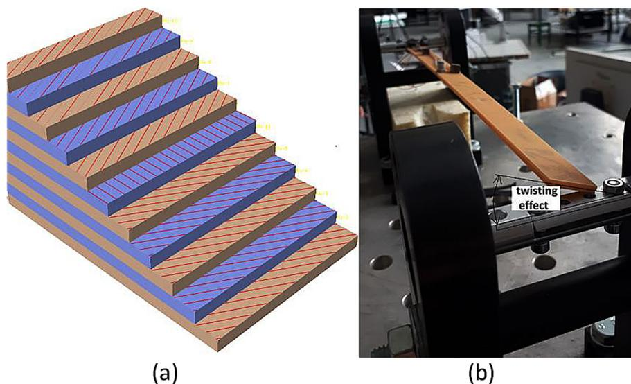
**Figure 5.** The stacking sequence set of composite beams (a) and the visible pre-twisting effect on the beam at asymmetric set of fibre layers (b)
