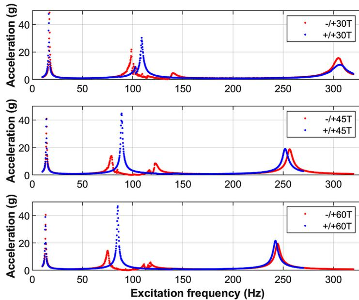
**Figure 6.** Amplitude – frequency response at the free end of the cantilever beam before exposition to temperature shocks of asymmetric (-/+) and symmetric (+/+) layer configurations for corresponding fiber sets 30°, 45° and 60°
