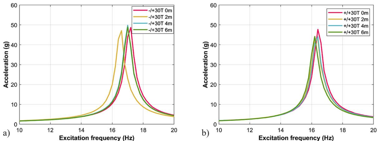
**Figure 7.** Amplitude – frequency response in with fibre set configuration 30°, exposed to temperature shocks in the vicinity of the first resonance zone of asymmetric (a) and symmetric (b) beams
