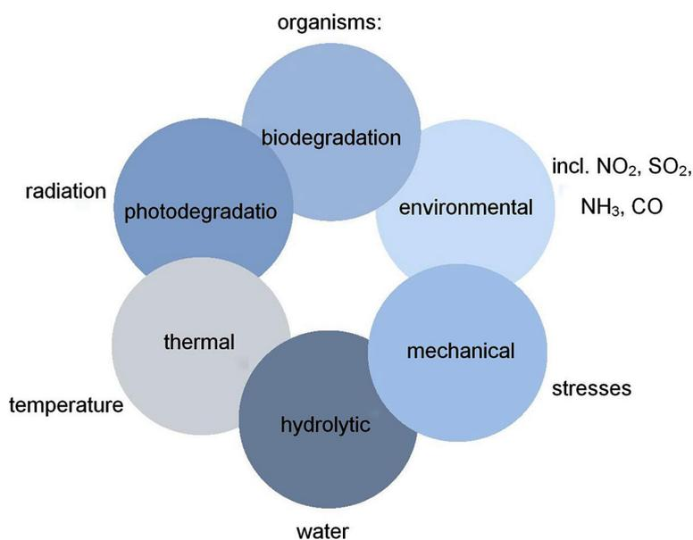
Figure 1. Factors affecting the degradation of polymeric materials (based on: [12])
