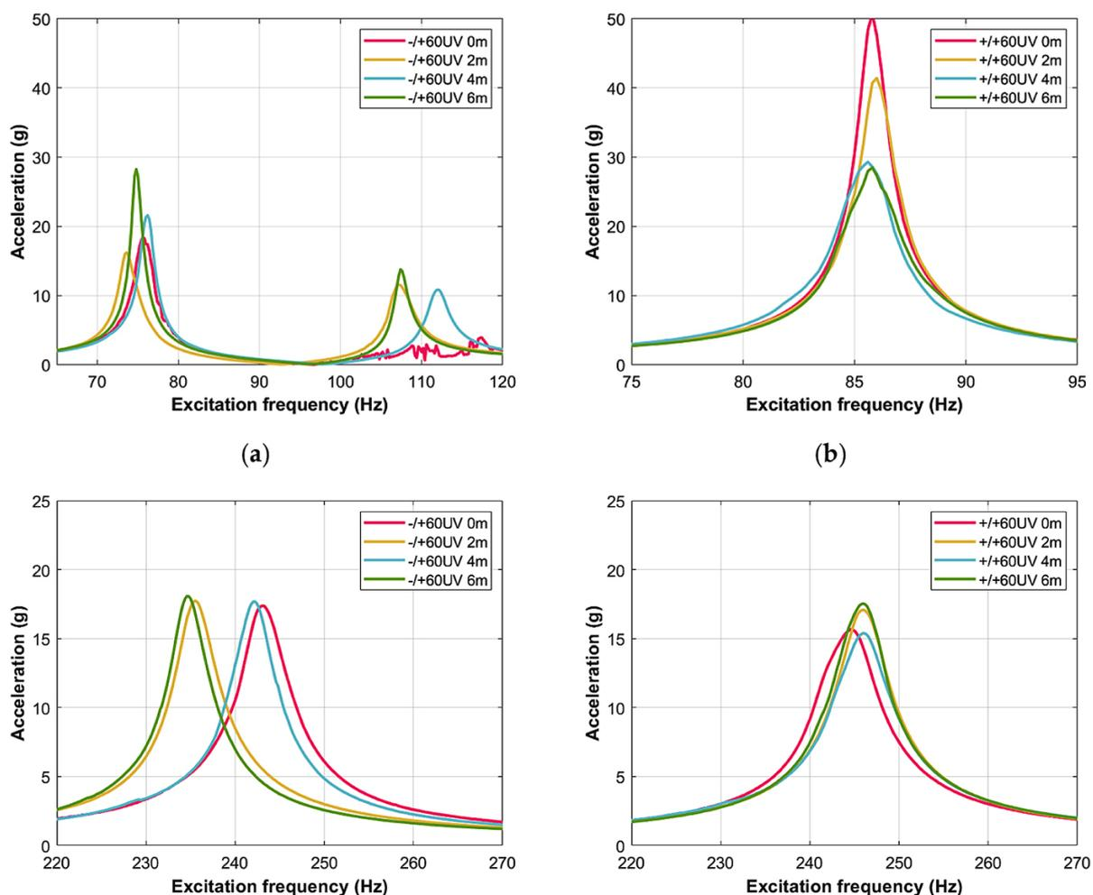
**Figure 12.** Amplitude – frequency responses of the cantilever beam with fibre set configuration 60°, exposed to UV radiation in the vicinity of the second (a, b) and the third (c, d) resonance zones, respectively
