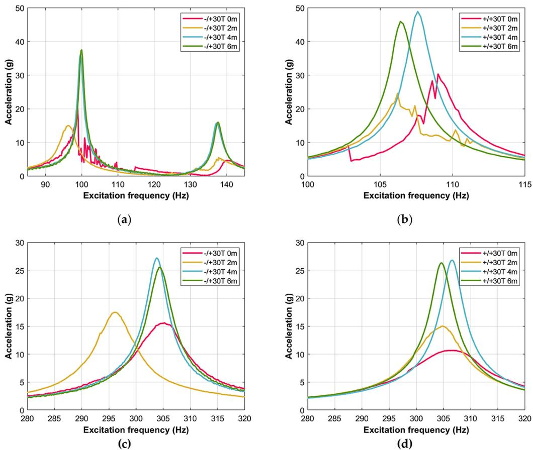
**Figure 8.** Amplitude – frequency responses of the cantilever beam with fibre set configuration  $30^\circ$ , exposed to temperature shocks in the vicinity of the second (a, b) and the third (c, d) resonance zones, respectively
