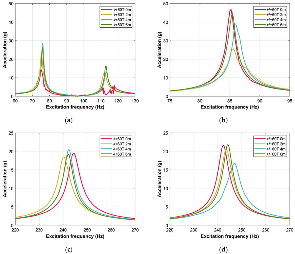
**Figure 9.** The amplitude – frequency responses of the cantilever beam with fibre set configuration  $60^\circ$ , exposed to temperature shocks in the vicinity of the second (a, b) and the third (c, d) resonance zones, respectively
