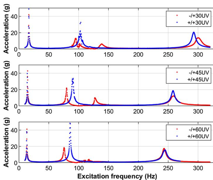
**Figure 10.** Amplitude – frequency response at the free end of the cantilever beam before UV radiation of asymmetric (-/+) and symmetric (+/+) layer configurations for corresponding fiber sets  $30^\circ$ ,  $45^\circ$  and  $60^\circ$
