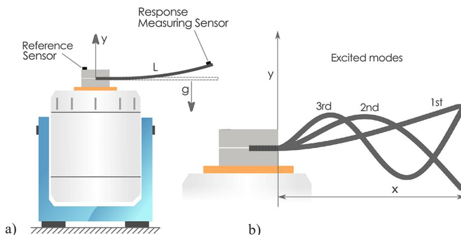
**Figure 4.** Schematic of the experimental stand of the electro dynamical shaker TIRAvib with positions of mounted accelerometers (a), the mode shapes excited during the dynamical tests (b)
