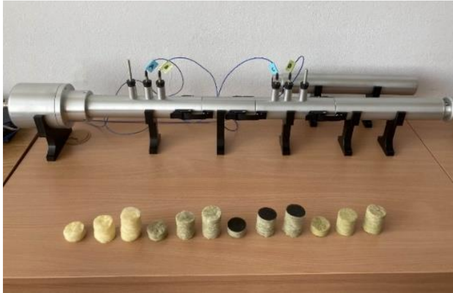
Fig. 1. Impedance tube with specimens of mineral wool of thickness 20, 40 and 50 mm and density (from the left): 25, 70, 110 and 150 kg/m 3 .
