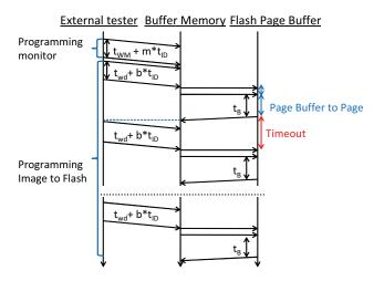
Fig. 2. Time flow in hybrid online mode of ISP
