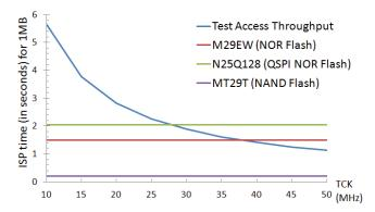
Fig. 6. Test access path throughput comparison with programming time of various Flash devices
