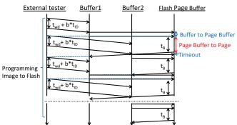
Fig. 4. Time flow in double-buffer hybrid online mode of ISP
