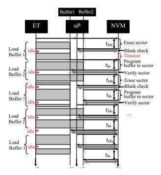
Fig. 7. Flow of ISP processes in double buffered hybrid online technique
