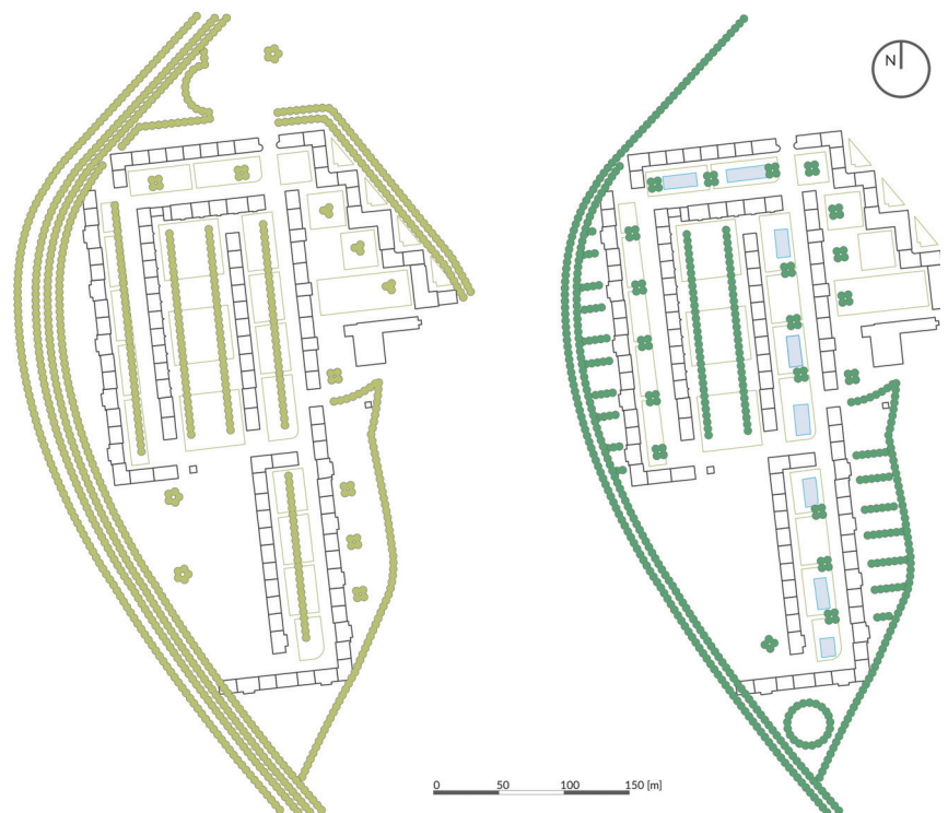
Fig. 1. The original spatial development plan by Paul Heim and Albert Kempter of 1928 (on the left) juxtaposed with real plantings made in the 40s' of the 20th century (on the right). The retention basins, existing in the same place until today, are marked with blue squares
