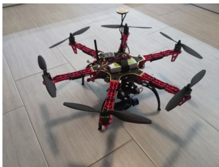
Figure 1. VTOL with structural elements printed using 3D printer (fot. Rafał Szymaniuk, WAT )
