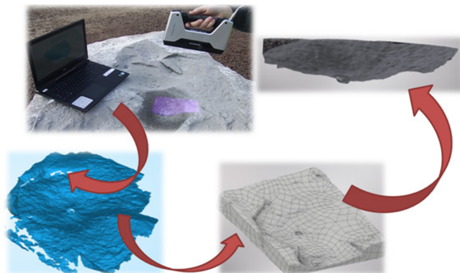
Figure 10: Scheme of processing the scans of rocks surfaces after their loosening.
