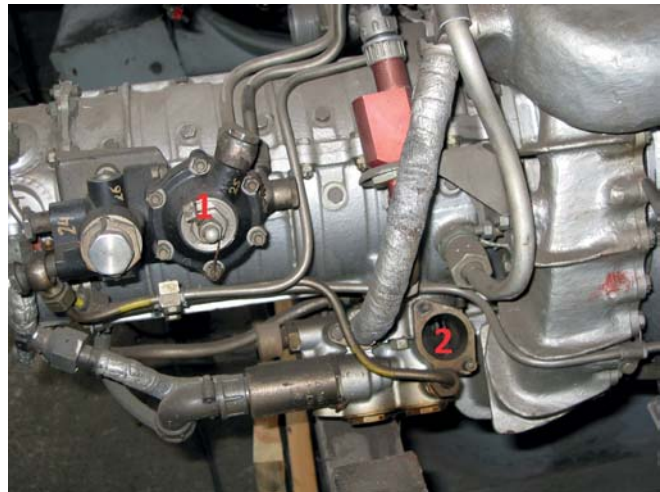
Photo 1. Air extraction from behind 6 th stage of the compressor 1. Air-extraction automatic controller; 2. Anti-surge valve.
