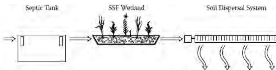
Fig. 13. Deep flow wetland and septic waste treatment; source: KADLEC and WALLACE [2009], modified
