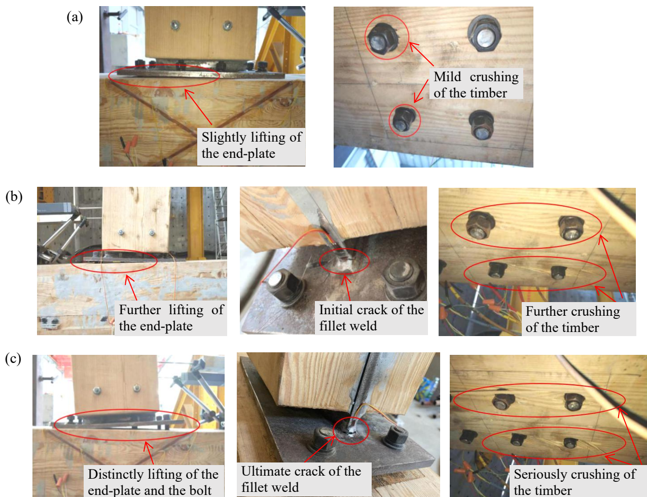
Fig.5. Failure phenomenons of JT joint: (a)Failure phenomenon when the displacement was 15mm;(b)Failure phenomenon when the displacement was 33mm;(c)Failure phenomenon when the displacement was 61mm.
