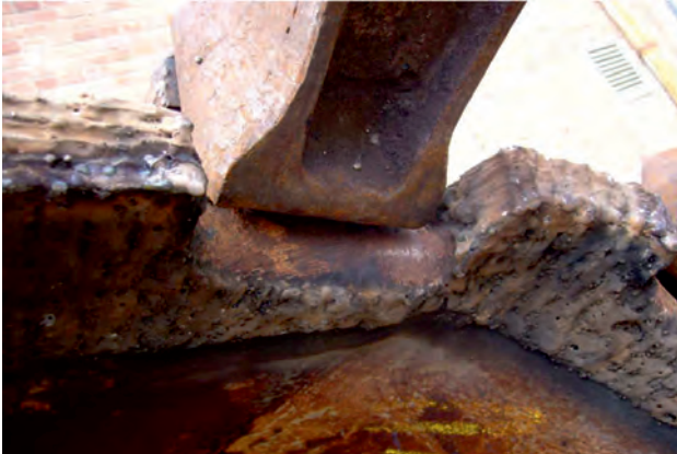
Fig. 3. The deficiency of the relative position of the tooth on cutting blade at the renewed buckets
