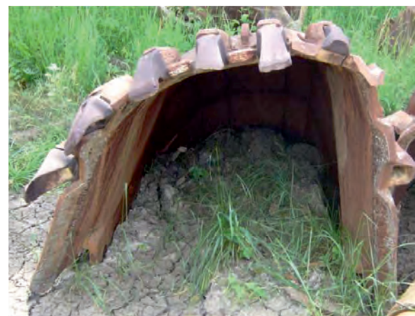
Fig. 7. Failure of teeth
