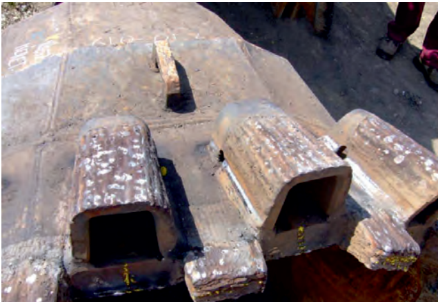
Fig. 6. Renewed cutting blade with adapters
