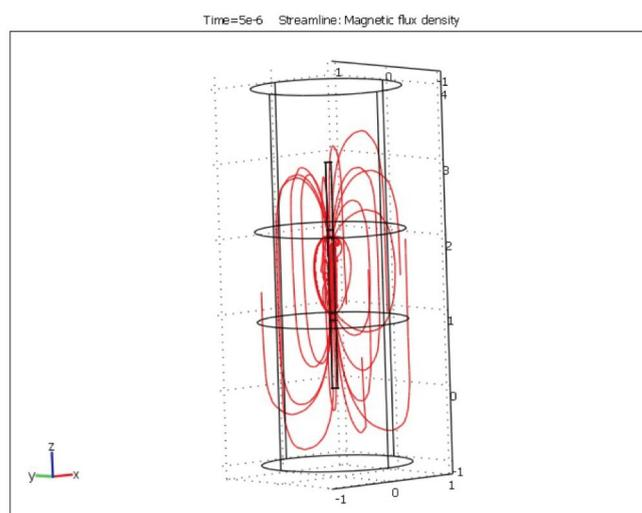
Fig. 3. The magnetic flux density lines around the sample ( $3 \text{ m} \times 0.01 \text{ m}$ ). The source is the magnetization that follows the form of stress shock wave. Modelling with Comsol multiphysics ®
