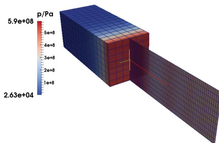
Fig. 6. The coupled model for 3D and 2D wave equation. The percussive shock is applied to the 2D side of the model. The speed of the travelling wave is 5000 m/s and the frequency of the applied pressure is 400 Hz
