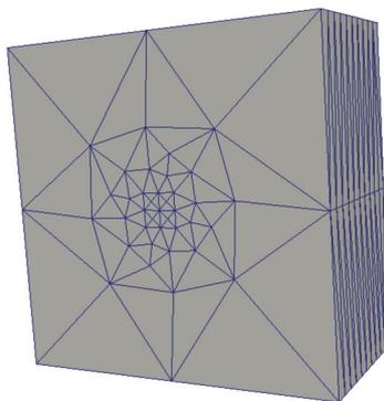
Fig. 1. The mesh of the finite element model for wave equation and eddy current model.
