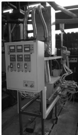
Fig. 1. Thermal reclaimer on the experimental stand in the Faculty of Foundry Engineering, AGH.
