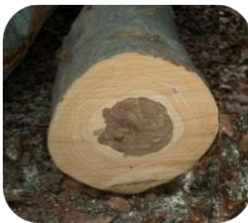
Fig. 1 View of the frontal cut of a beech wood with a false heartwood.
