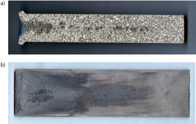
Fig. 2. Macrostructure of permanent mould cast ingot (specimen 1) (a) and high pressure die casting (specimen 2) (b)
